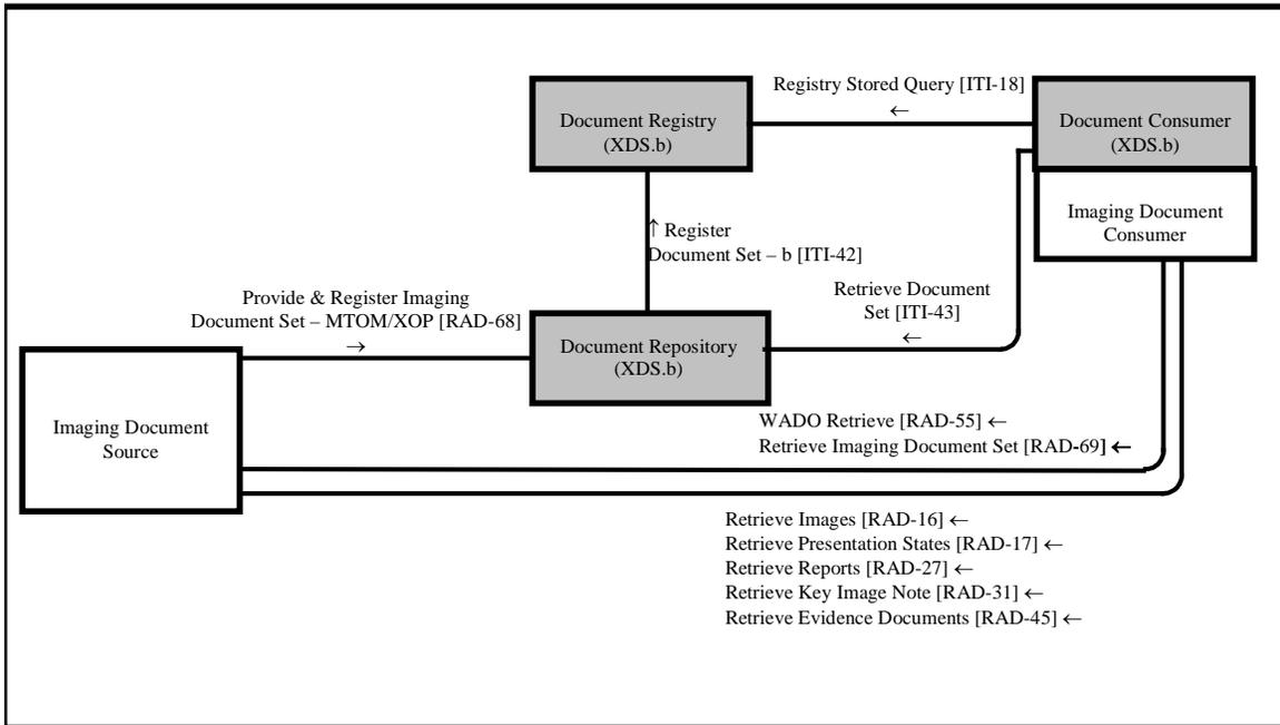
**Figure 18.1-1: Cross-Enterprise Document Sharing for Imaging Diagram**
