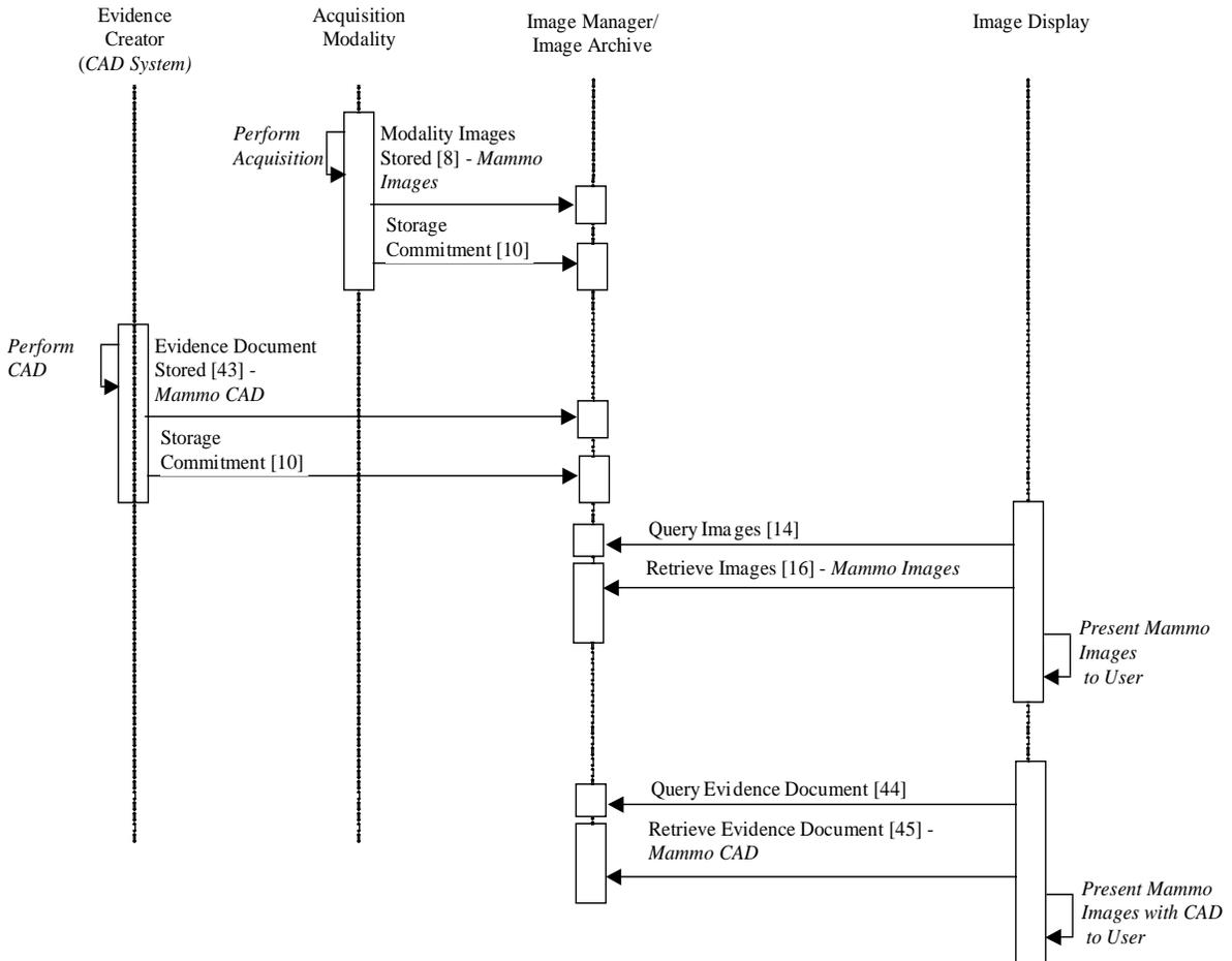
**Figure 19.3-1: Basic Process Flow in Mammography Image Profile**
