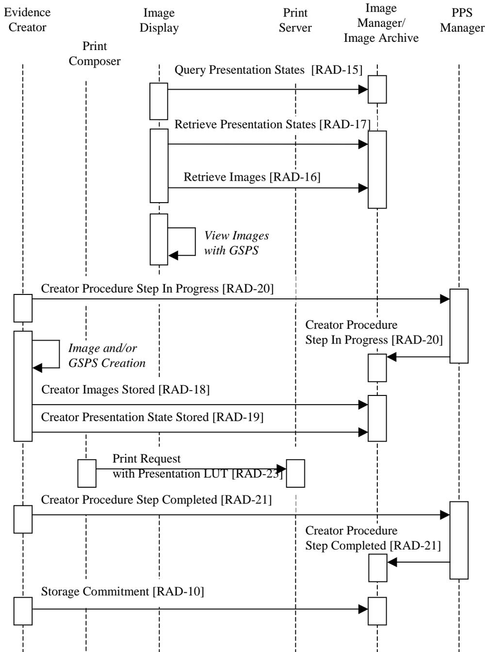
Figure 5.3-1: Consistent Presentation of Images Process Flow
