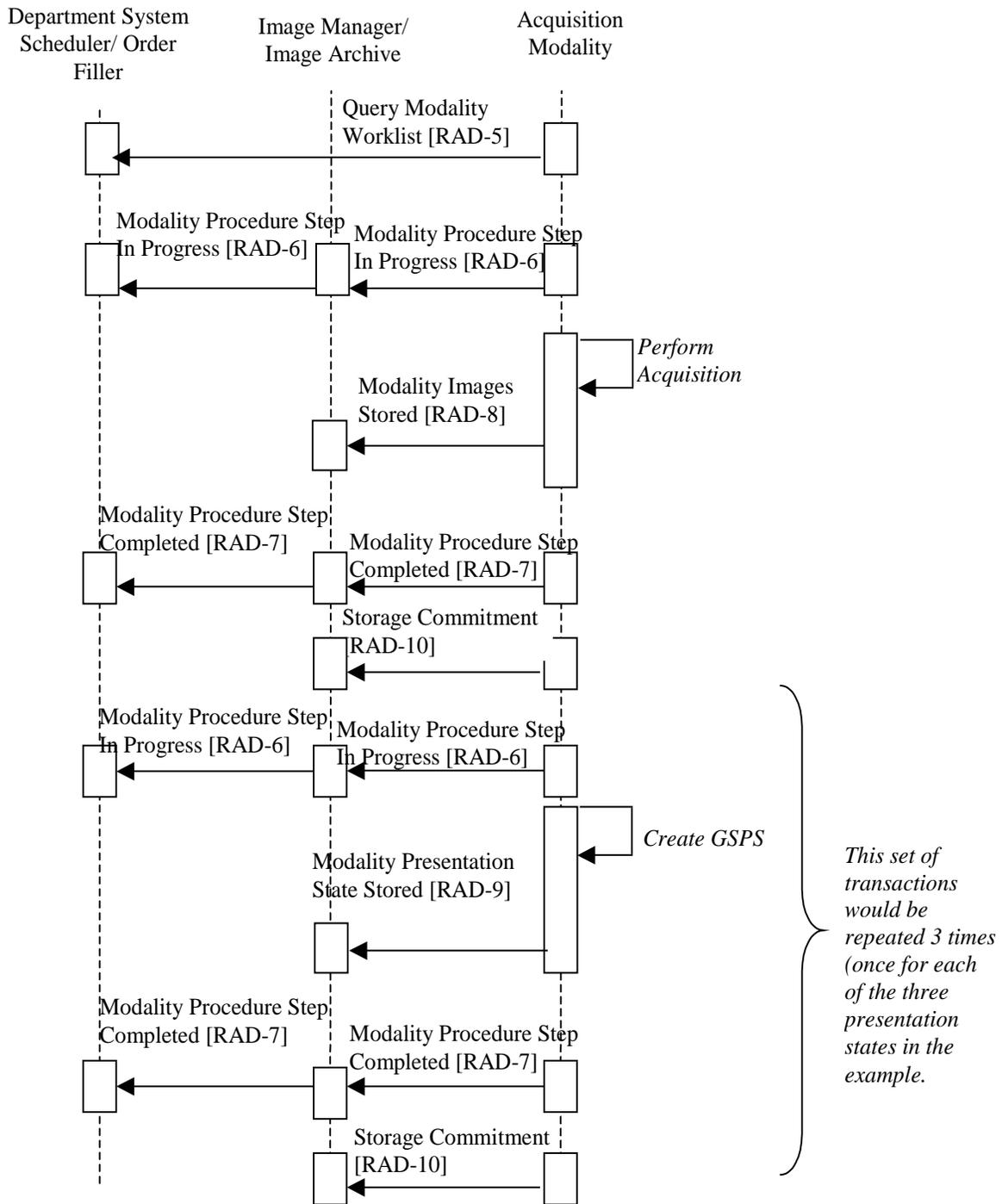
**Figure 6.3-1: Presentation of Grouped Procedures Process Flow**
