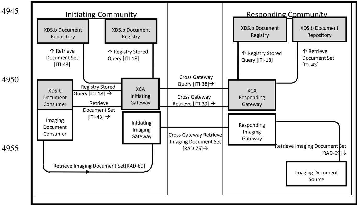
**Figure 29.1-1: Cross-Community Access for Imaging Actor Diagram**
