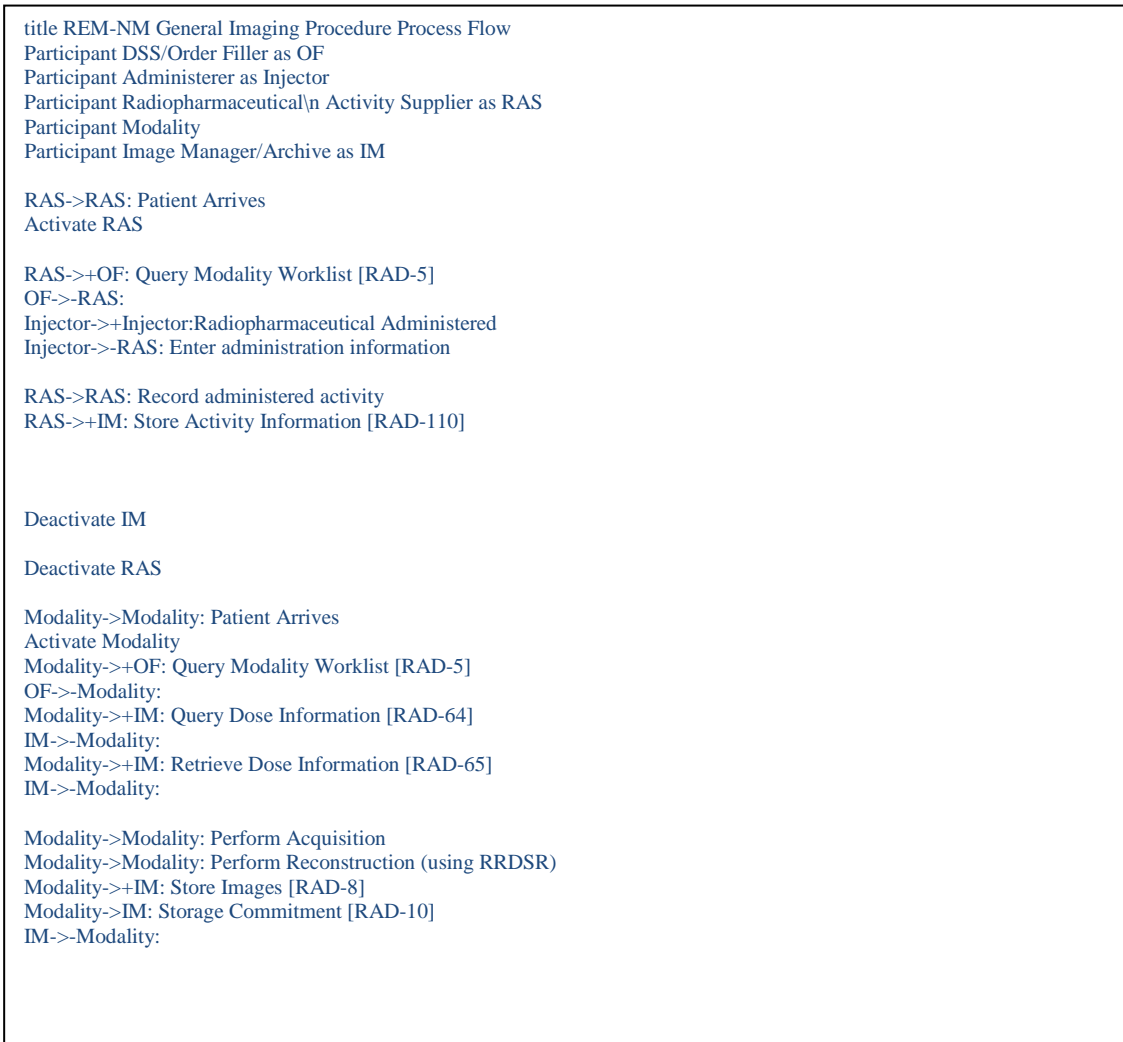
Figure 40.4.2.2-2: Diagram Pseudocode for General Imaging Procedure Process Flow
