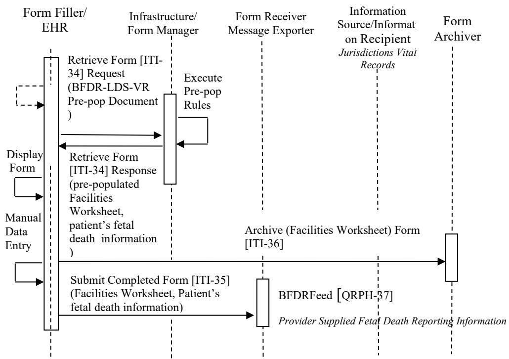
**Figure X.4.2.1.3-1: Use Case 1 - Forms Data Capture with Messaging**
