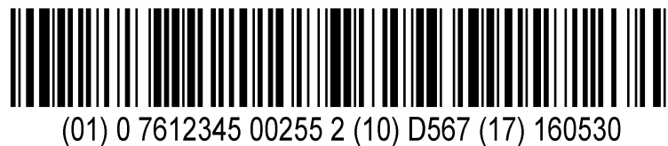
Figure 8: GS1-128 barcode representing, GTIN, batch/lot and expiry date
