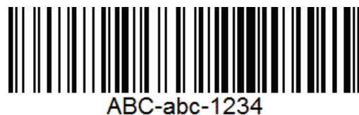
Figure 5: Example of a Code 128 barcode
