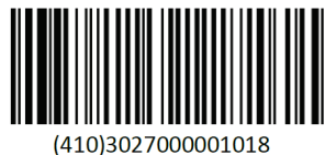
Figure 9: GS1-128 carrying Ship to - Deliver to Global Location Number: AI (410) with GLN
