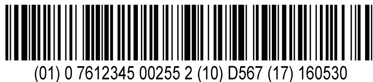
945 Figure 8: GS1-128 barcode representing, GTIN, batch/lot and expiry date
