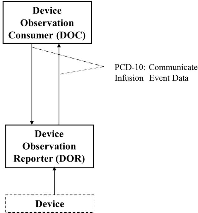
**Figure X.1-1: Infusion Pump Event Communication Actor Diagram**
