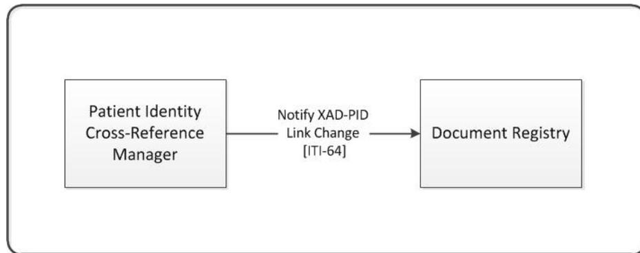
**Figure 31.1-1: XAD-PID Change Management Profile Actor Diagram**
