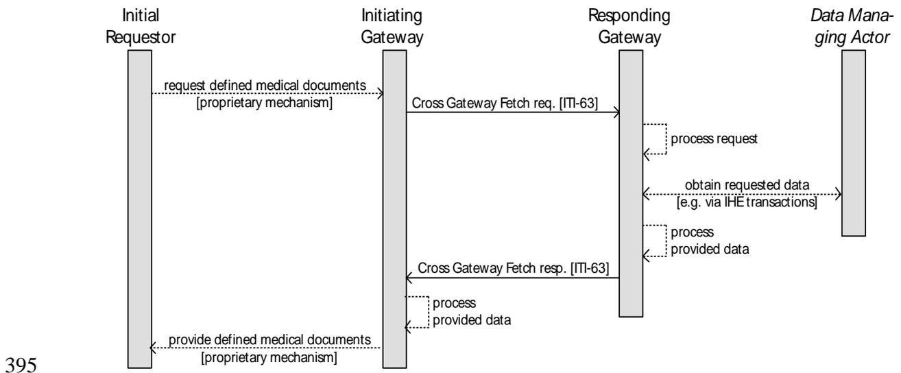
**Figure 29.4.2-1: Basic Process Flow in XCF Profile**
