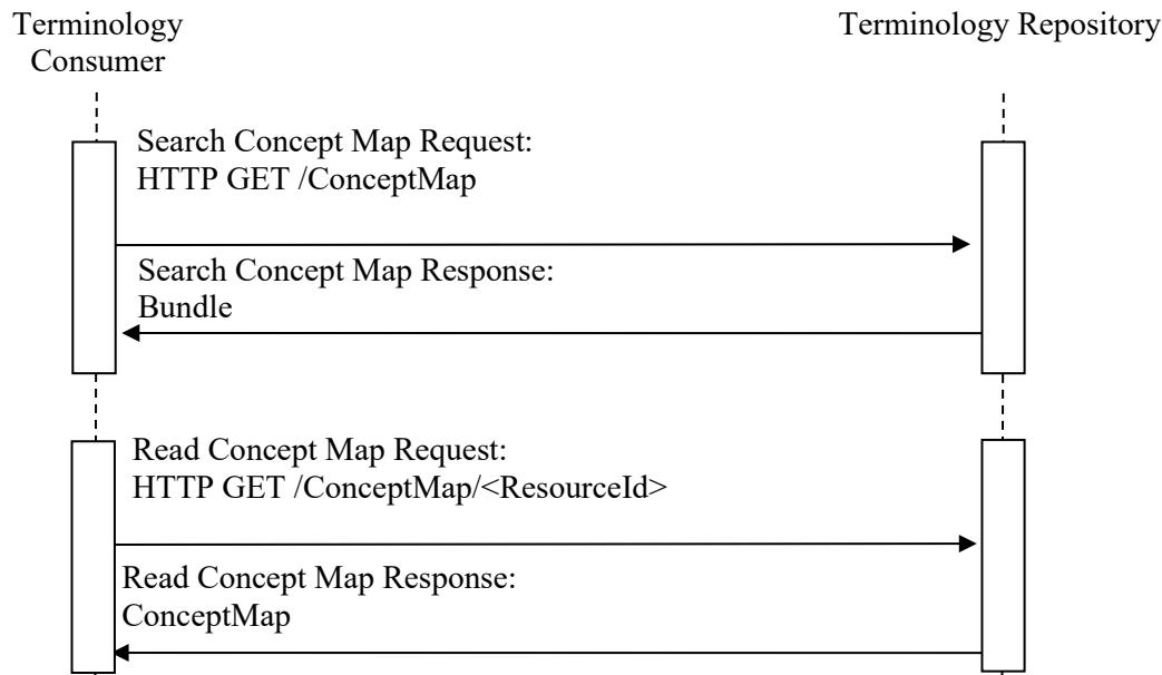
**Figure 3.100.4-1: Interaction Diagram**
