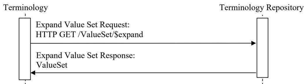
**Figure 3.97.4-1: Interaction Diagram**
