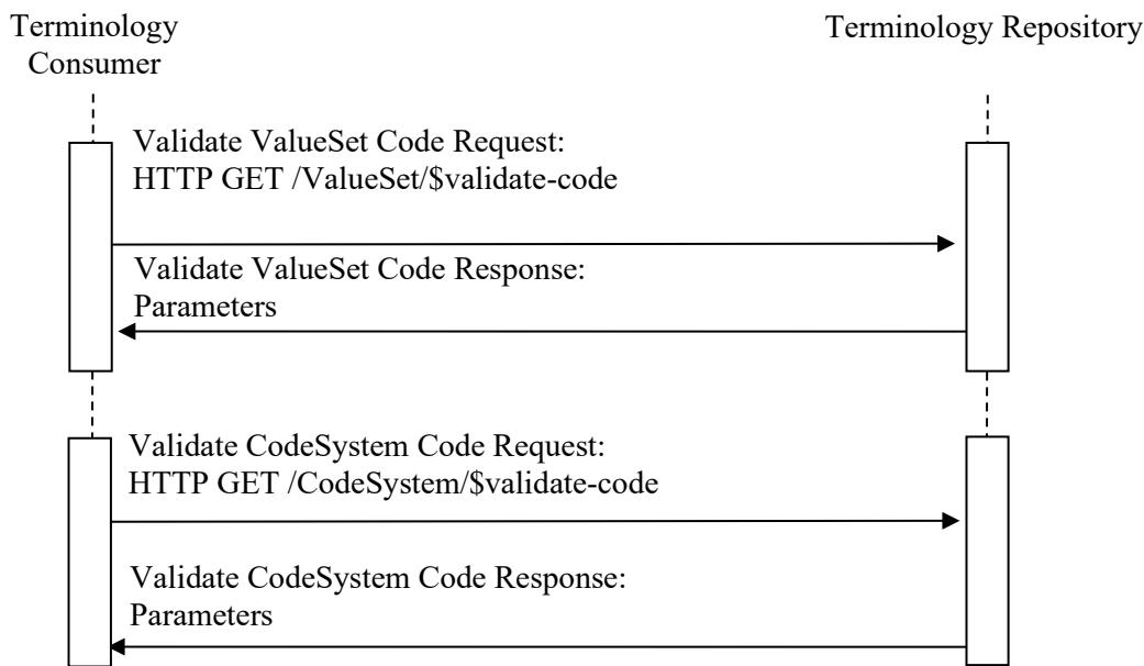
**Figure 3.99.4-1: Interaction Diagram**
