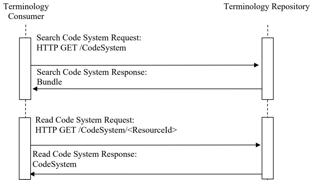
**Figure 3.96.4-1: Interaction Diagram**
