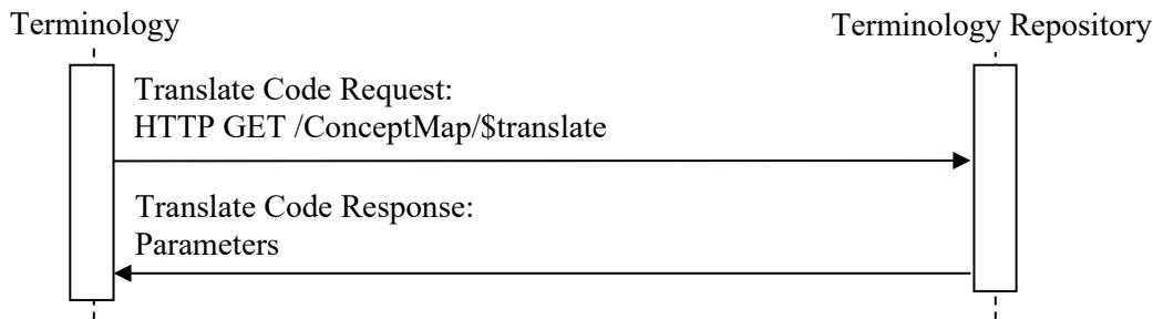
**Figure 3.101.4-1: Interaction Diagram**
