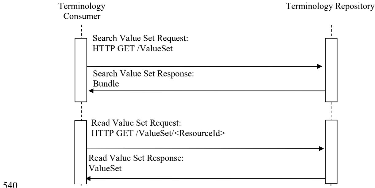
Figure 3.95.4-1: Interaction Diagram
