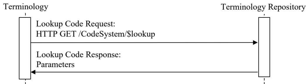
**Figure 3.98.4-1: Interaction Diagram**
