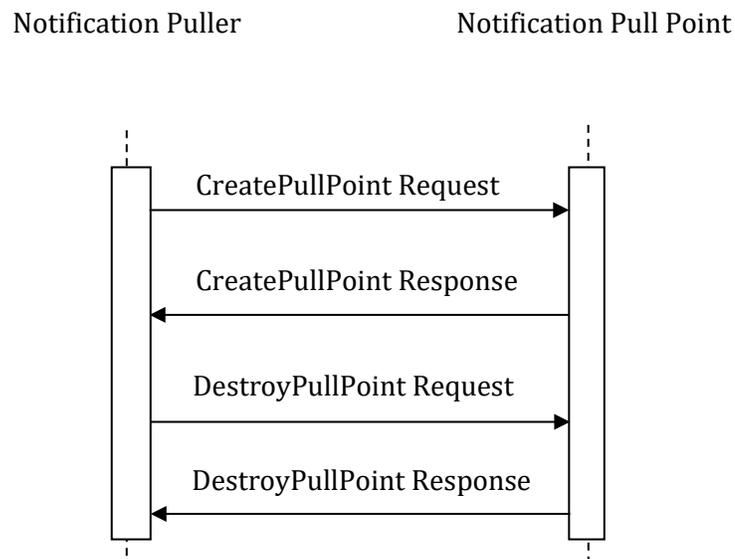
**Figure 3.69.4-1: Interaction Diagram**
