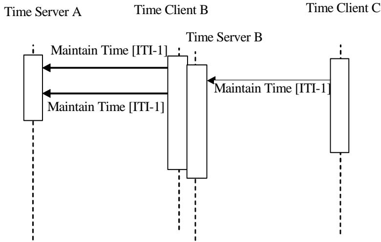
**Figure 7.3-1 Basic Process Flow in Consistent Time Profile**
