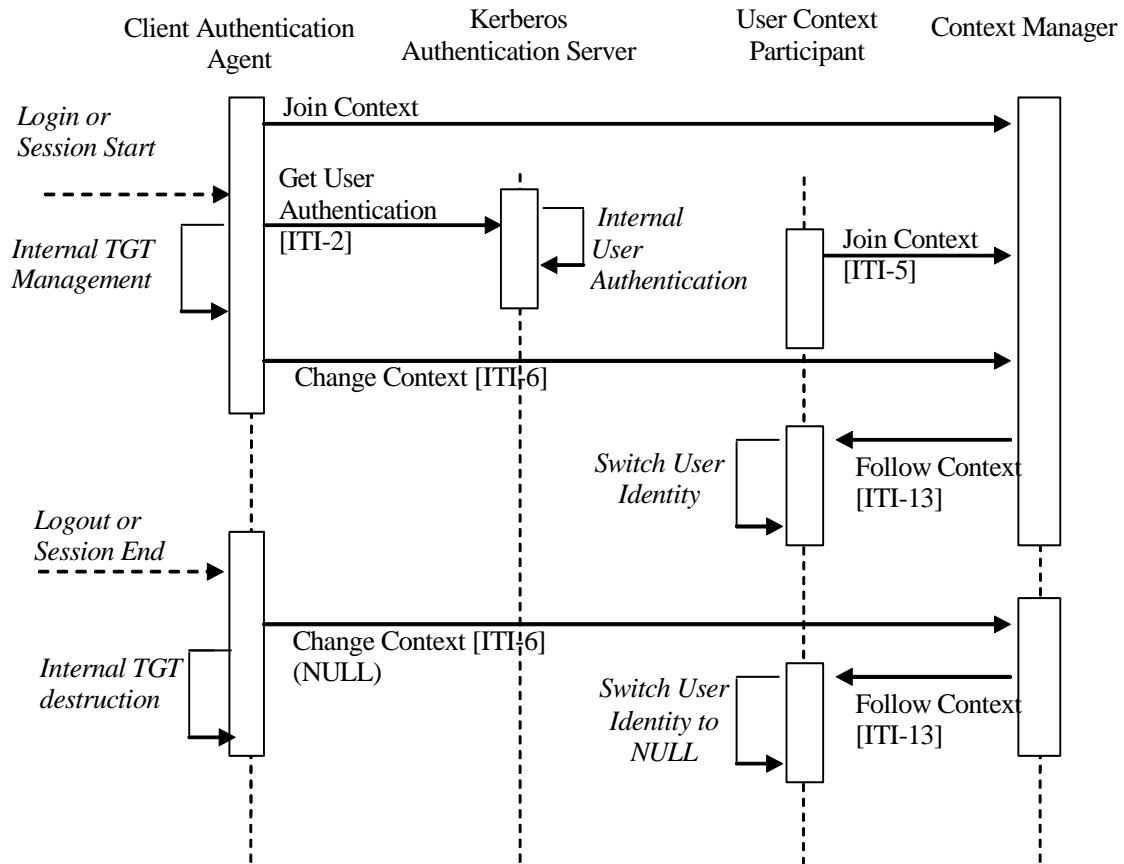
**Figure 4.3.2-1 Process Flow with User Synchronized Applications**
