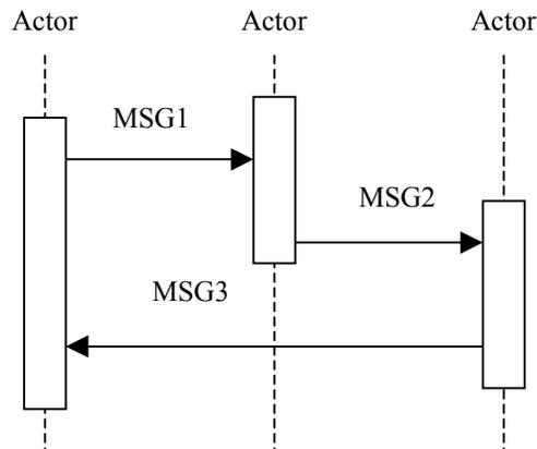
255 The interaction diagrams used in the IHE Technical Framework are modeled after those described in Grady Booch, James Rumbaugh, and Ivar Jacobson, *The Unified Modeling Language User Guide*, ISBN 0-201-57168-4. Simple acknowledgment messages are omitted from the diagrams for brevity.
