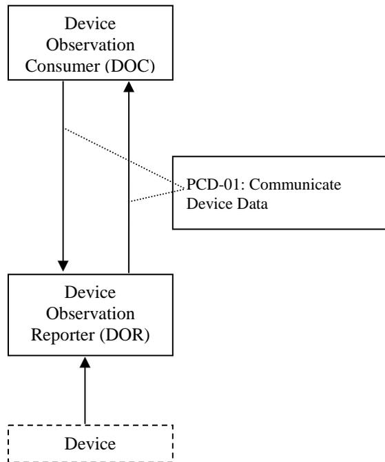
**Figure 3.1-1: DEC Integration Profile with Actors and Transactions**
