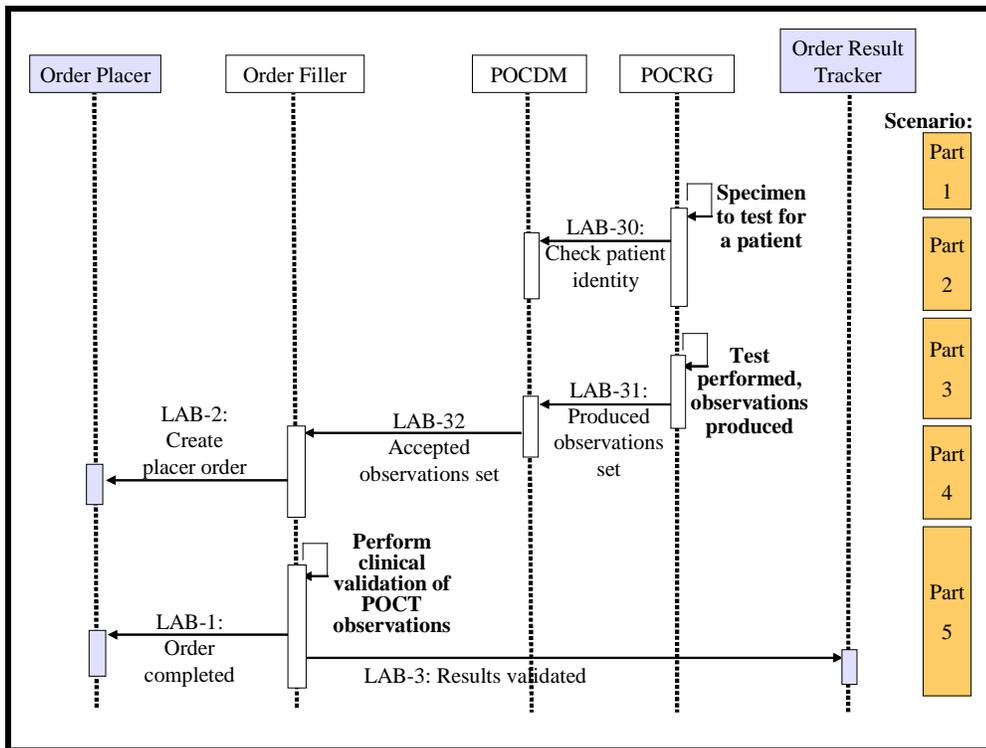
Figure 6.7.2-1: Process flow for use case 6.4.2
