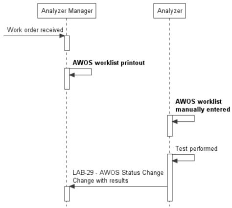
Figure X.6.4-1: Normal process with AWOS manual entry
