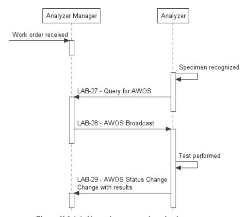
Figure X.6.1-1: Normal process when Analyzers query
