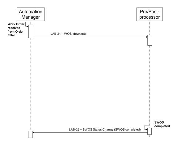
Figure 5.2.1-1: Process Flow for WOS downloaded before specimen arrival
