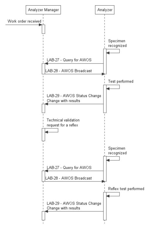
Figure X.6.9-1: Reflex decided on the Analyzer Manager at the technical validation time
