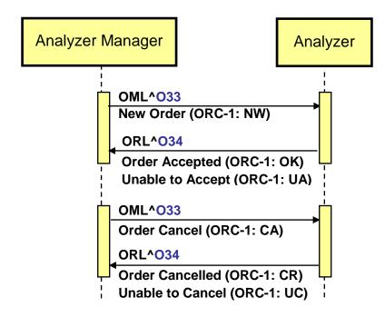
Figure 3.R.4-1: AWOS management on Analyzer in broadcast mode
