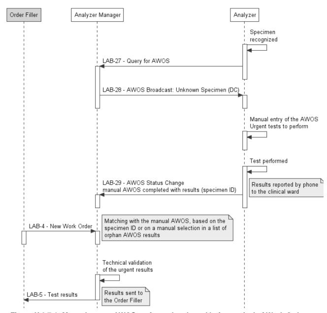
Figure X.6.7-1: Manual urgent AWOS performed and used before arrival of Work Order
