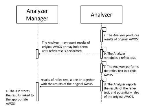
Figure X.6.8-1: Reflex decided on the Analyzer immediately after first run
