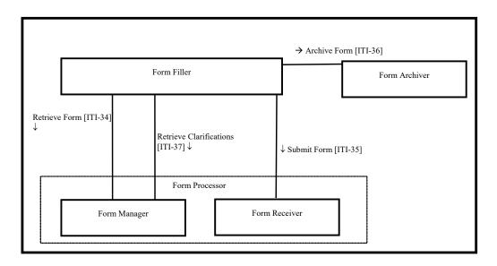
Figure 17.2-1: Retrieve Form for Data Capture Actor Diagram
