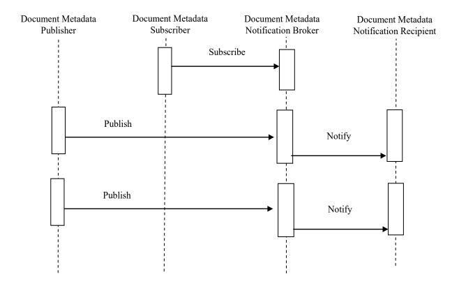
Figure 26.4.2.2.2-1: Interaction Diagram for Long-term Subscription Use Case
