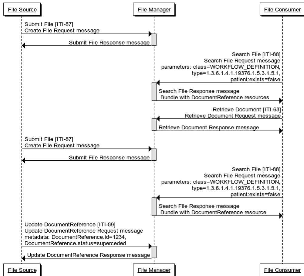
Figure 47.4.2.2.2-1: Basic Process Flow in NPFSm Profile for Workflow Definition Documents management
