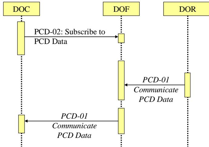
Figure 5 Subscribe to PCD Data Interaction Diagram
