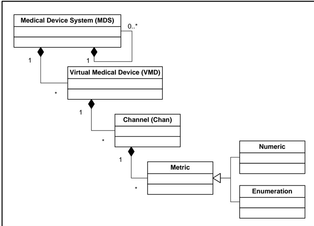
**Figure 9 Basic ISO/IEEE 11073 Containment Tree**
